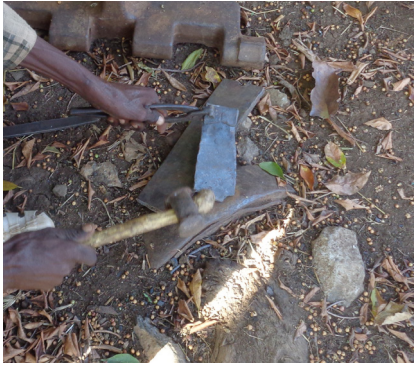
FIGURE 17 Demonstration of usage of blacksmithing tools: a metal rod held over an anvil with a tong and struck with a hammer, Aṭeyä (B. Kribus/V. Krebs)
